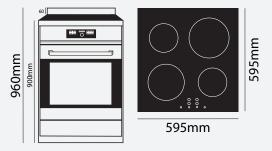
Introducing Parmco's first Induction Freestanding Stove. An induction cooktop works by using magnetic energy to heat cookware, essentially turning the cookware into its own source of heat – the induction system is highly efficient, allowing for a rapid rise or drop in temperature providing faster cooking times.
